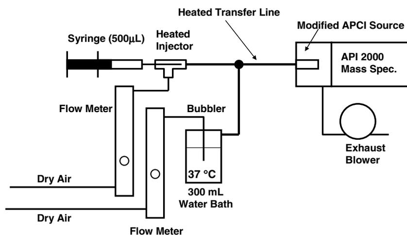
**Figure 2.** Final VOC dilution set-up designed for partial humidification of the airflow. VOC is injected using a syringe into a heated injector to ensure efficient vaporization. The syringe flow rate is controlled using a syringe pump.
