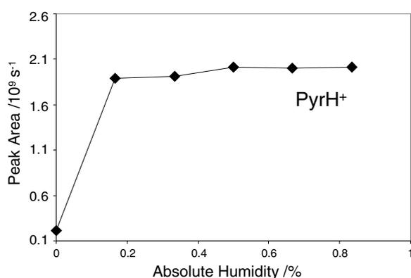
**Figure 9.** Measured signal response of protonated pyridine in APCI-MS as a function of absolute humidity. The increase in signal is dramatic at low absolute humidities, but the signal quickly plateaus. The pyridine concentration is 50 ppb.
