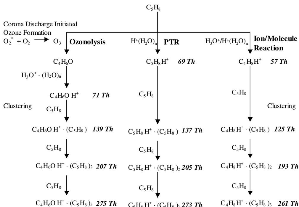
**Figure 7.** Overview of the isoprene ion/molecule reactions proposed to occur in the APCI ion source. Ozone is formed by oxygen excitation at the corona discharge needle.
