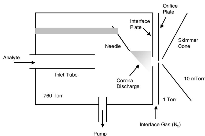
**Figure 1.** Basic schematic of the modified APCI source employed for gas analysis.
