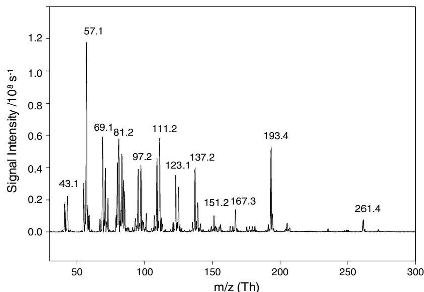
**Figure 6.** APCI-MS of 800 ppb isoprene showing the richness of the ion/molecule chemistry occurring in the source region of the instrument.
