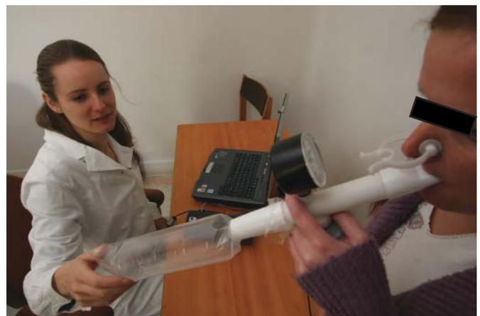
**FIGURE 1.** Sampling of exhaled breath for smellprint analysis by electronic nose. The subject inhales through a volatile organic compound filter and exhales with stable flow rate against resistance.
